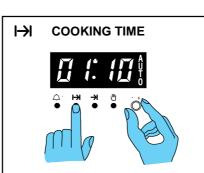
Press button C and while turning knob A enter the required cooking time. Auto will appear on the right hand side of the clock, select the required temperature and oven function. When cooking is completed an audible signal will be heard for approx 2 mins. To cancel press button B and return control and thermostat knobs to 'O' OFF.
